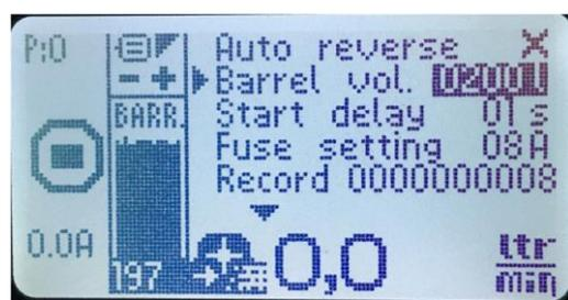
**Auto reverse** - This function start automatically reverses. The pump stops automatically when the hoses are exhausted.
