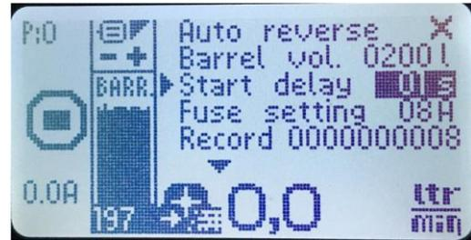
**Pump stop if flow is lower than 0,5 U/min.**
