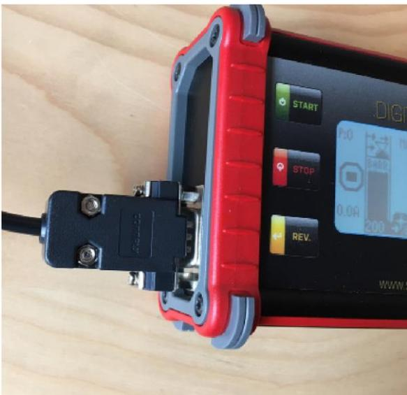
*If the machine gives a 12 V signal (most cutters), the blue cable is connected to +12 V. Cuttecs gives signal 12 V after putting down pick up, start drums and machine is moving*
